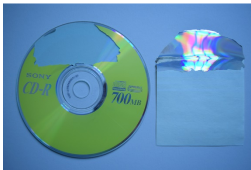
Information layer removed from a CD by the adhesive on a post-it note
